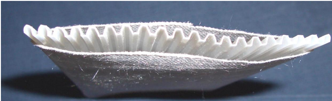
Fig. 7 Photo of the wick drain used for the project
